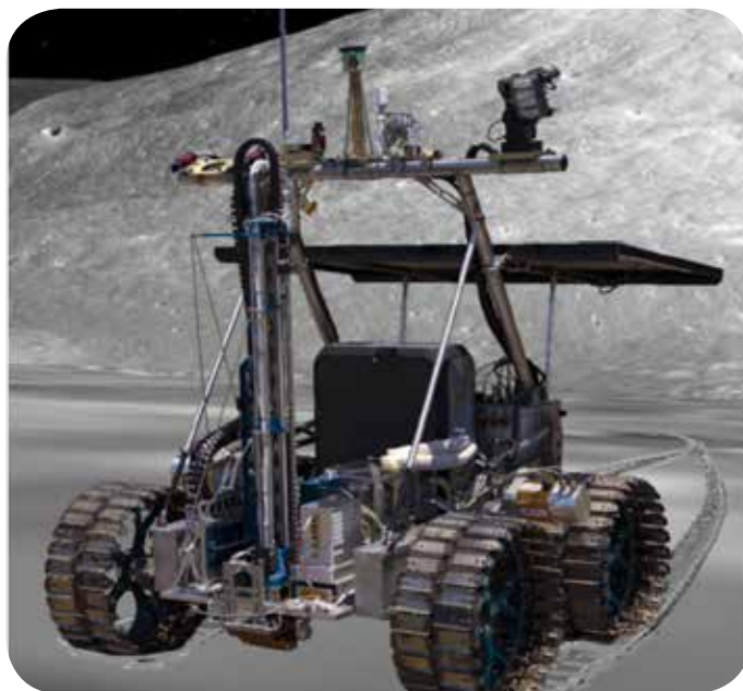
The RESOLVE payload concept shown prospecting for volatiles in a polar region of the Moon.
