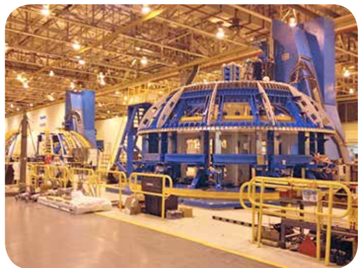
The Circumferential Dome Weld Tool, located at NASA's Michoud Assembly Facility in Louisiana, will be used to create the SLS core stage domes out of 12 panels.
